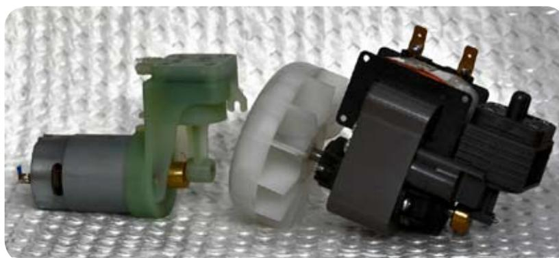
The photograph above shows a pump from a cheap machine on the left and a pump from a Lava machine on the right. The pump on the left is based on a generic motor which is made in China and weights 270 grams. The Lava pump is made in Germany especially for Landig and weights over 1200 grams.
